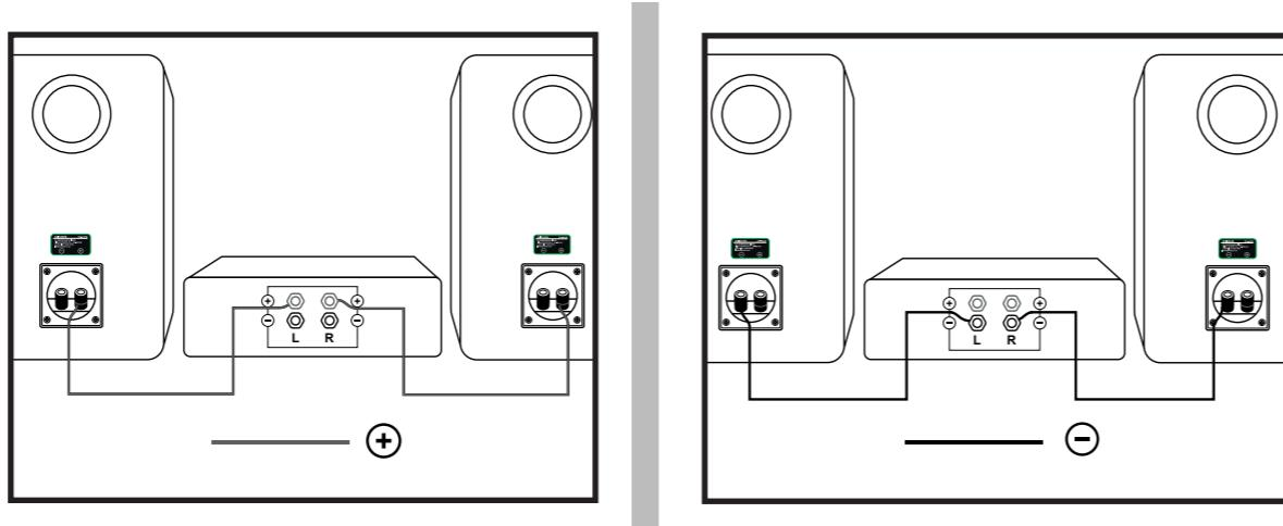
Connect the positive of the speaker with the positive of the amplifier (respect the polarity)
